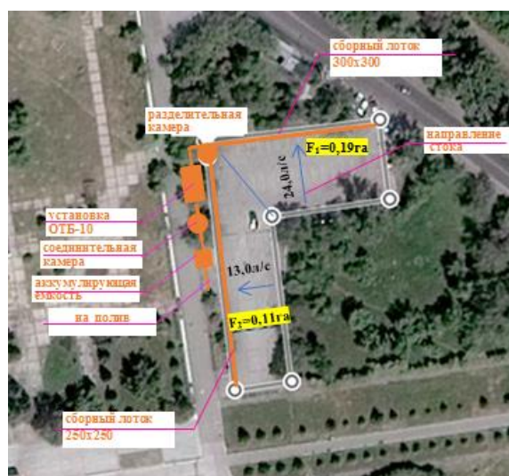
Parking plan with surface water treatment plants
