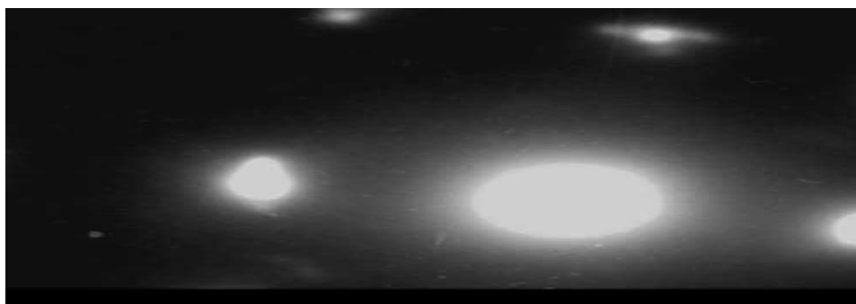
Figure 21. Microdiffraction pattern (a) obtained from a grain section of fragmented ferrite and its indexed scheme (b)
