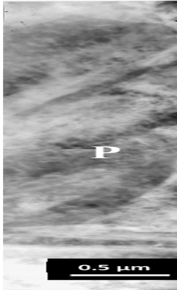
Figure 23. Electron microscopic image of the fine structure of the surface of a grade two steel sample after electrolytic plasma surface quenching: packet-plate martensite, the boundary of two grains (P – packet martensite, LLM – Lamellar low-temperature martensite)
