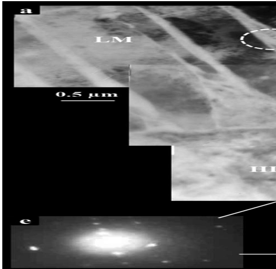
Figure 6. Electron microscopic image of the fine structure of the sample surface after electrolyte-plasma surface hardening obtained by transmission electron microscope
