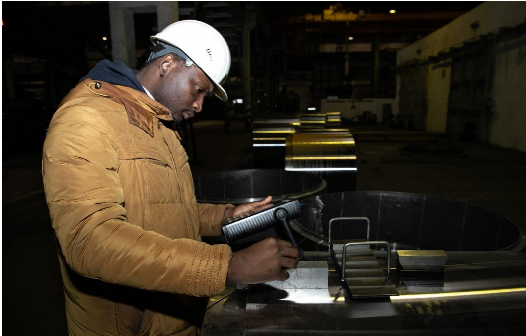
Figure 2- Research and development work of ultrasonic inspection Currently, the methods of ultrasonic inspection of forgings, castings are standardized [3], and a large number of NC instructions have also been developed.
